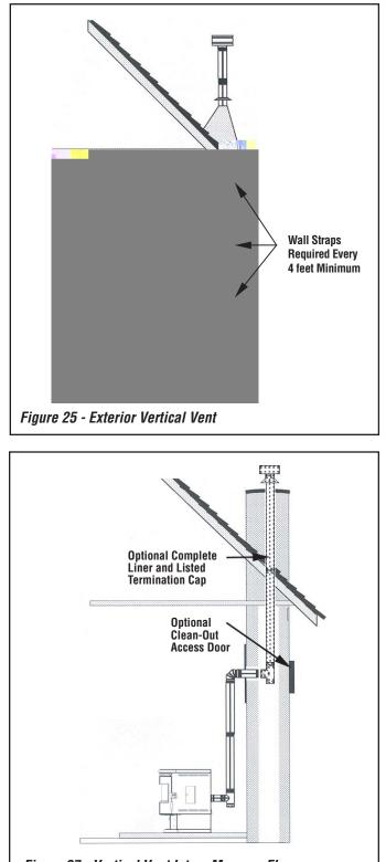
Figure 27 - Vertical Vent Into a Masonry Flue
